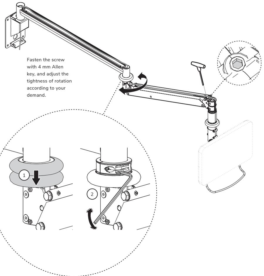
Fasten the screw with 4 mm Allen key, and adjust the tightness of rotation according to your demand.
