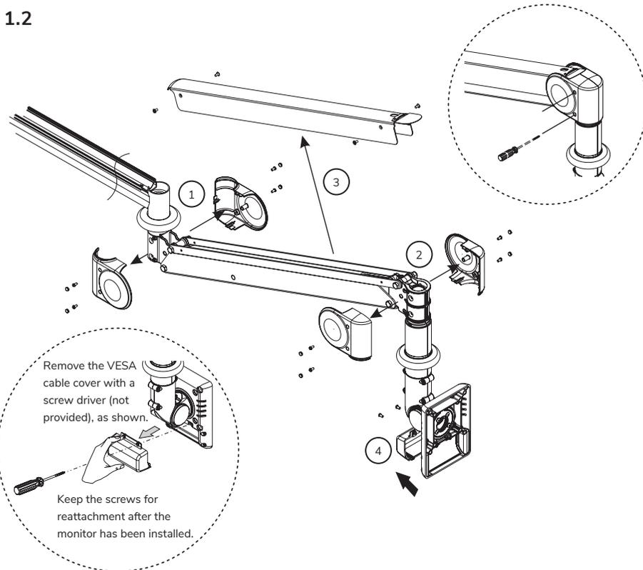
Remove the VESA cable cover with a screw driver (not provided), as shown.
