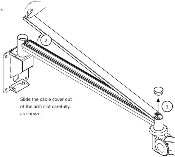
Slide the cable cover out of the arm slot carefully, as shown.
